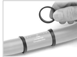
Pic 1: VRO Center Ring Removal: If these handlebars are to be used in a conventional stem, the two plastic centering rings in the center of the handlebar must be removed. To remove these easily, simply wrap a rag around the rings and press the end of the handlebar firmly against the ground. You may wish to place a piece of cardboard or some other softer material between the end of the bar and the ground to avoid the possibility of damaging the end of the handlebar.
